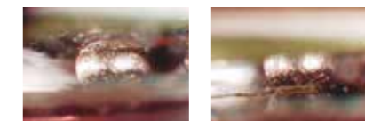
Points of contact for BGA upper parts. Points of contact for BGA lower parts.
