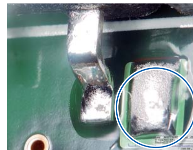
Picture 2: Normal flux residue as a result of proper flux activation to heat between land and leads.
