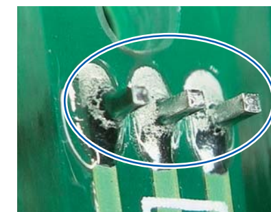
Picture 67: Heat dissipation from the pattern during manual soldering creates good gloss on the fillet.
