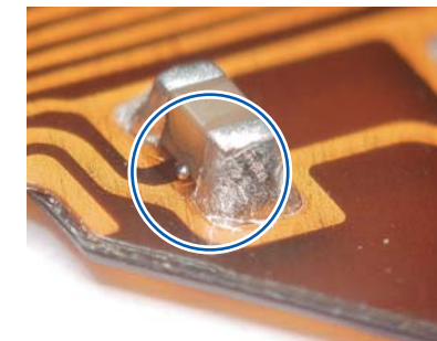
Picture 96: Image taken using a Rotary-Head Adapter (MX-5040RZ) Side balls from excessive solder printing
