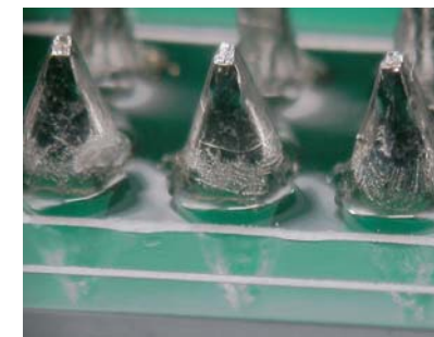
Picture 28: Residual flux stays on printed area of solder paste.
