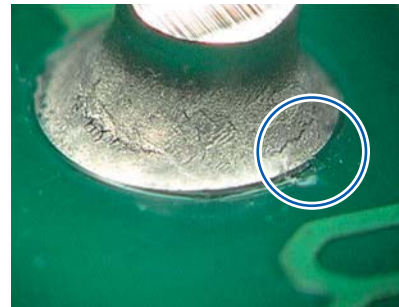
Picture 153: The small bubbles on the side of the fillet indicate the possibility of a void in the hole.
