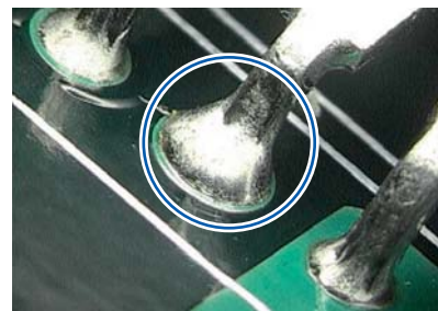
Picture 135: Good wetting with a multi-layer board
