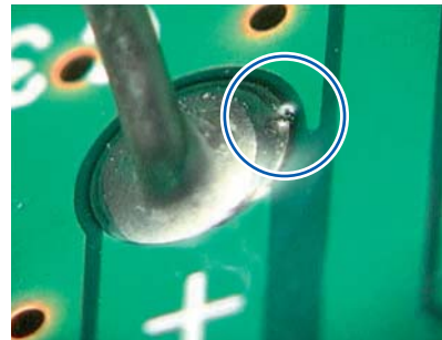
Picture 153: The small bubbles on the side of the fillet indicate the possibility of a void in the hole.
