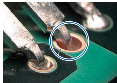
Picture 133: Insufficient through hole wetting
