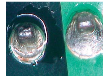
Picture 139: Lead surface is good
