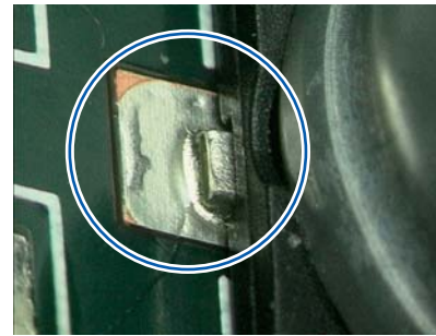
Picture 87: Replaced with bigger land
