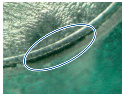
Picture 156: High solder well temperature causes land stripping
