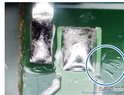
Picture 1: Spattered flux residue may cause poor wetting or create voids.
