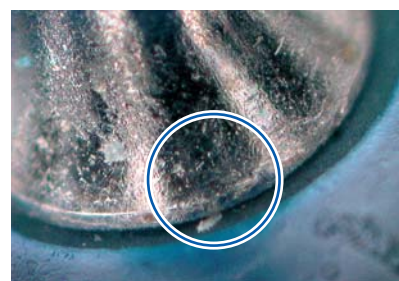
Picture 160: Land stripping and residual flux are visible on the bottom of the fillet.
