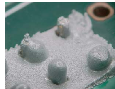
Picture 27: Solder reacts to heat on leads and no bridges are formed despite bold printing.
